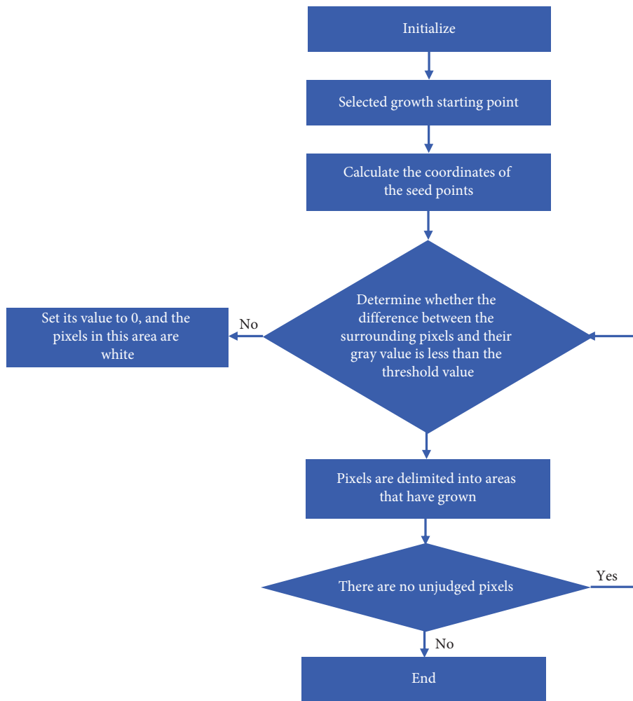
FIGURE 5: Segmentation flowchart based on the threshold region growing algorithm.
