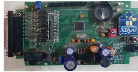
FIGURE 5: Hardware of PIC16f877a with Zigbee.
