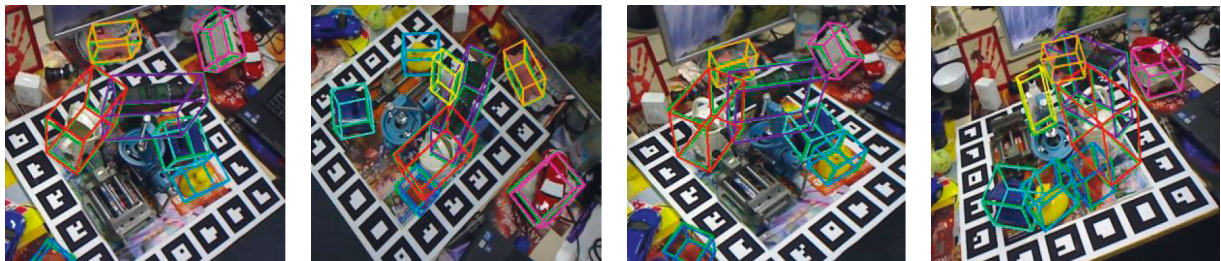
FIGURE 3: The qualitative results on the occlusion LINEMOD dataset. The green 3D bounding boxes around the objects show the ground truths, and the other colors show the proposed system’s predictions.
