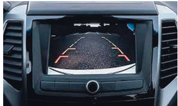
FIGURE 7: Reverse assistance LCD [26].
