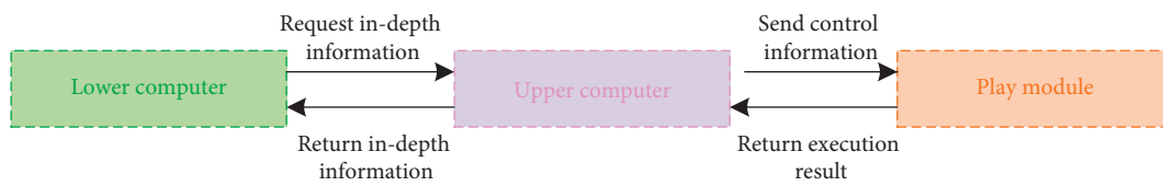
FIGURE 6: The architecture of the gesture recognition module.
