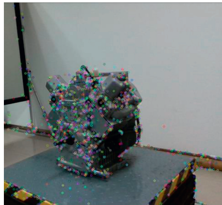
FIGURE 4: SIFT method diesel engine feature extraction results.
