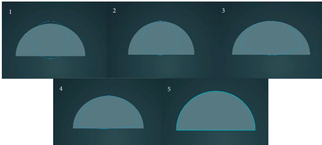
FIGURE 3: The segmentation effect of the optimized image segmentation model on the artificially synthesized noise map. 1–5 were the original image and contour lines, those after 15 steps of evolution, those after 45 steps of evolution, those after 65 steps of evolution, and those after 95 steps of evolution.
