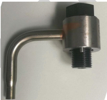
FIGURE 7: Actual photo of the nozzle.
