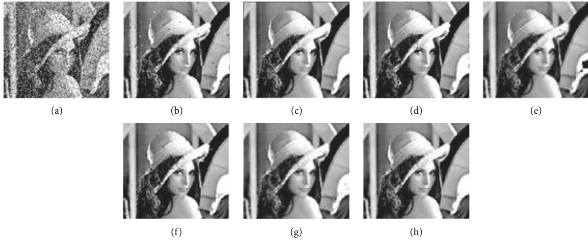
FIGURE 4: Results of the proposed and standard methods when the image is corrupted with 30% noise density: (a) Original image with 30% noise density; (b) MF [8]; (c) AMF [9]; (d) IQR [15]; (e) AIQR [16]; (f) BPDF [28]; (g) NAFSM; and [13] (h) EBD.
