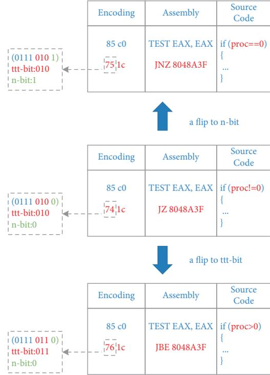
FIGURE 12: Example of flips in ttt-bit and n-bit in the Jcc instruction.
