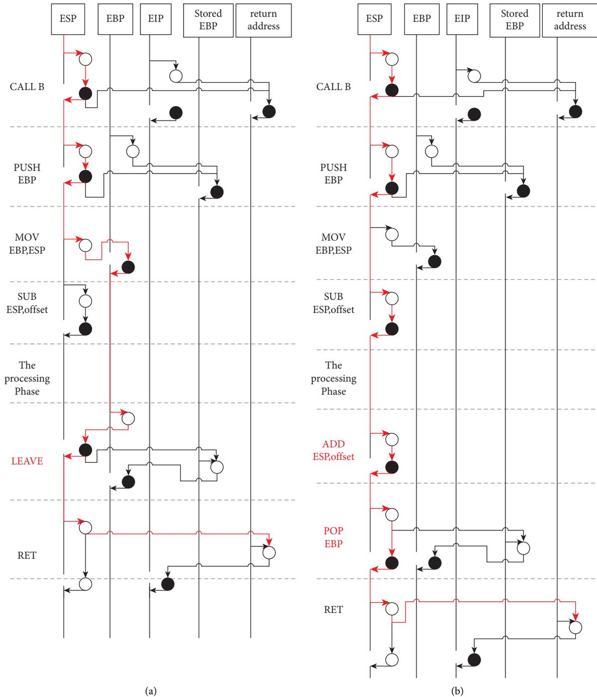
FIGURE 11: A snippet of typical assembly code of a call to procedure. (a) LEAVE-way restoring. (b) ADD-way restoring.
