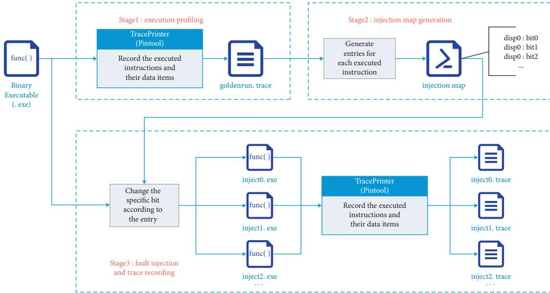
FIGURE 1: Workflow of fault injection experiment.
