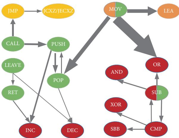
FIGURE 10: Instruction class mutations due to a bit flip in the opcode field (number of cases  $\geq 50$ ). Green node denotes call-related instructions. Yellow node denotes control transfer instructions. Orange node denotes data transfer instructions. Red node denotes arithmetic instructions.
