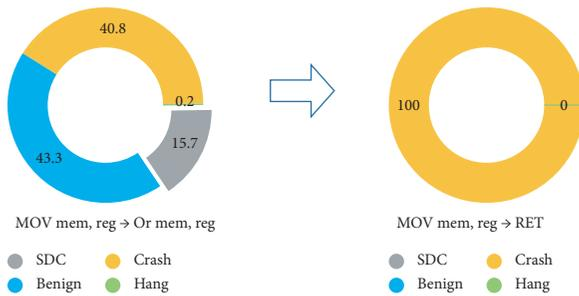
FIGURE 17: Results for the injections on the most significant bit of opcode field of MOV instruction under old encoding scheme and new encoding scheme.
