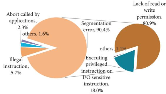
FIGURE 6: Distribution of crash causes for realigned cases.
