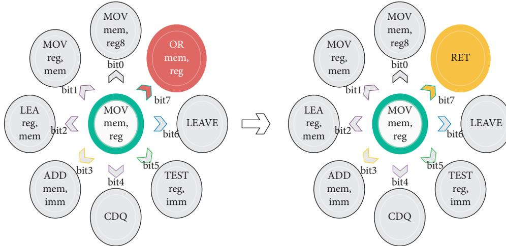
FIGURE 16: Neighboring encodings of MOV mem, reg in the old encoding scheme and new encoding scheme.
