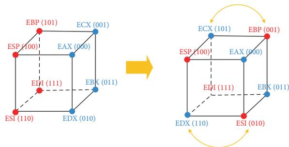
FIGURE 15: Hamming space of the original and redesigned reg field encodings.
