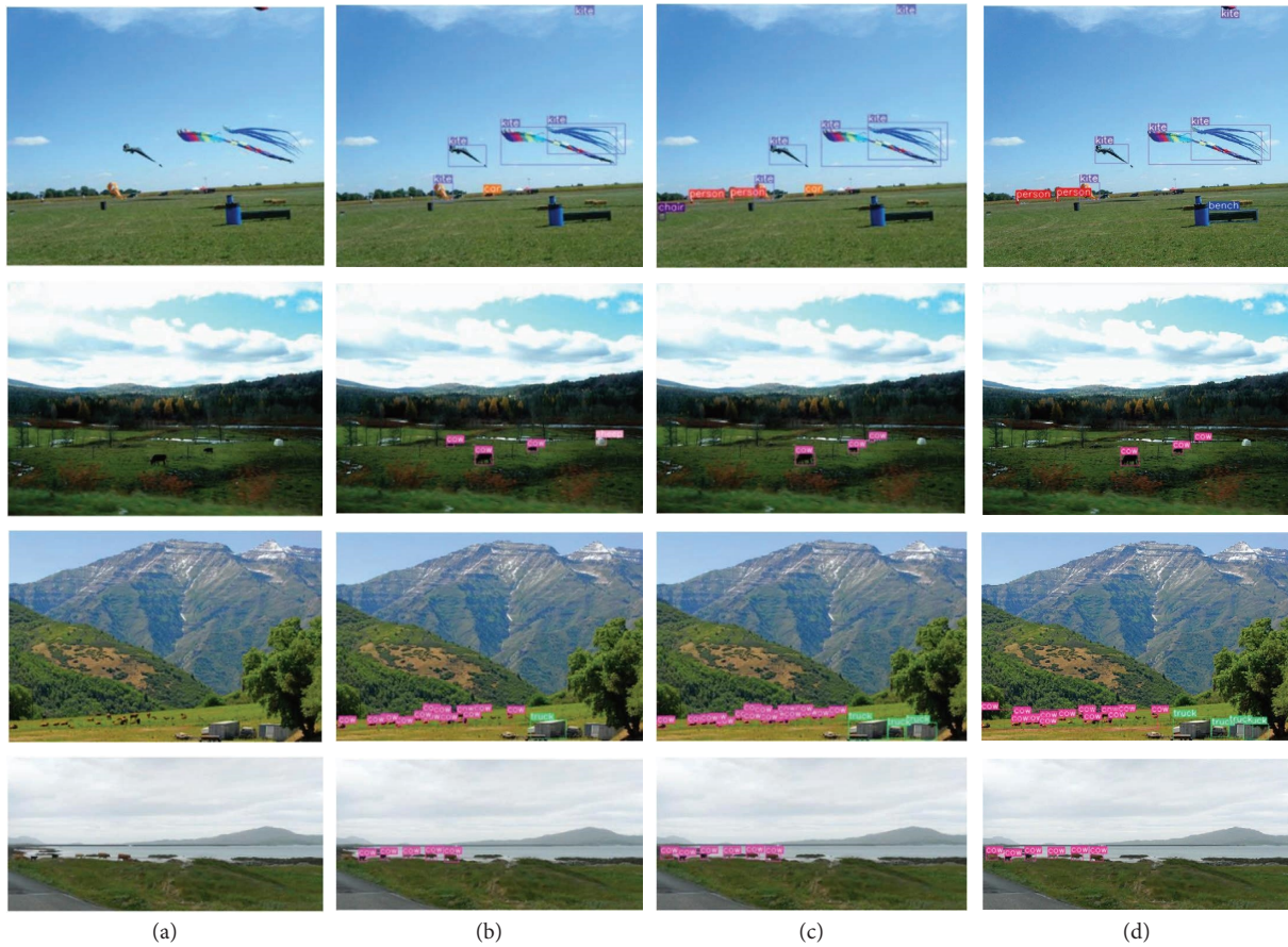
FIGURE 8: Comparisons of small object detection results. (a) The original images; (b) RetinaNet test results; (c) MFEFNet test results; and (d) the ground truth.
