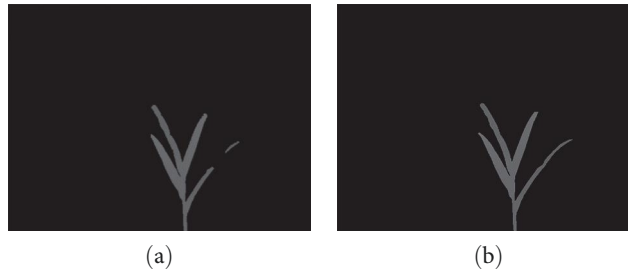
FIGURE 7: Comparison of hole-filling effect in-depth image: (a) depth image by mean filter; (b) depth image by improved mean filter.
