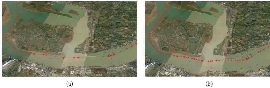
FIGURE 8: Comparison between the unrepaired and repaired trajectories: (a) the trajectory before AIS repairing and (b) the trajectory after AIS repairing.
