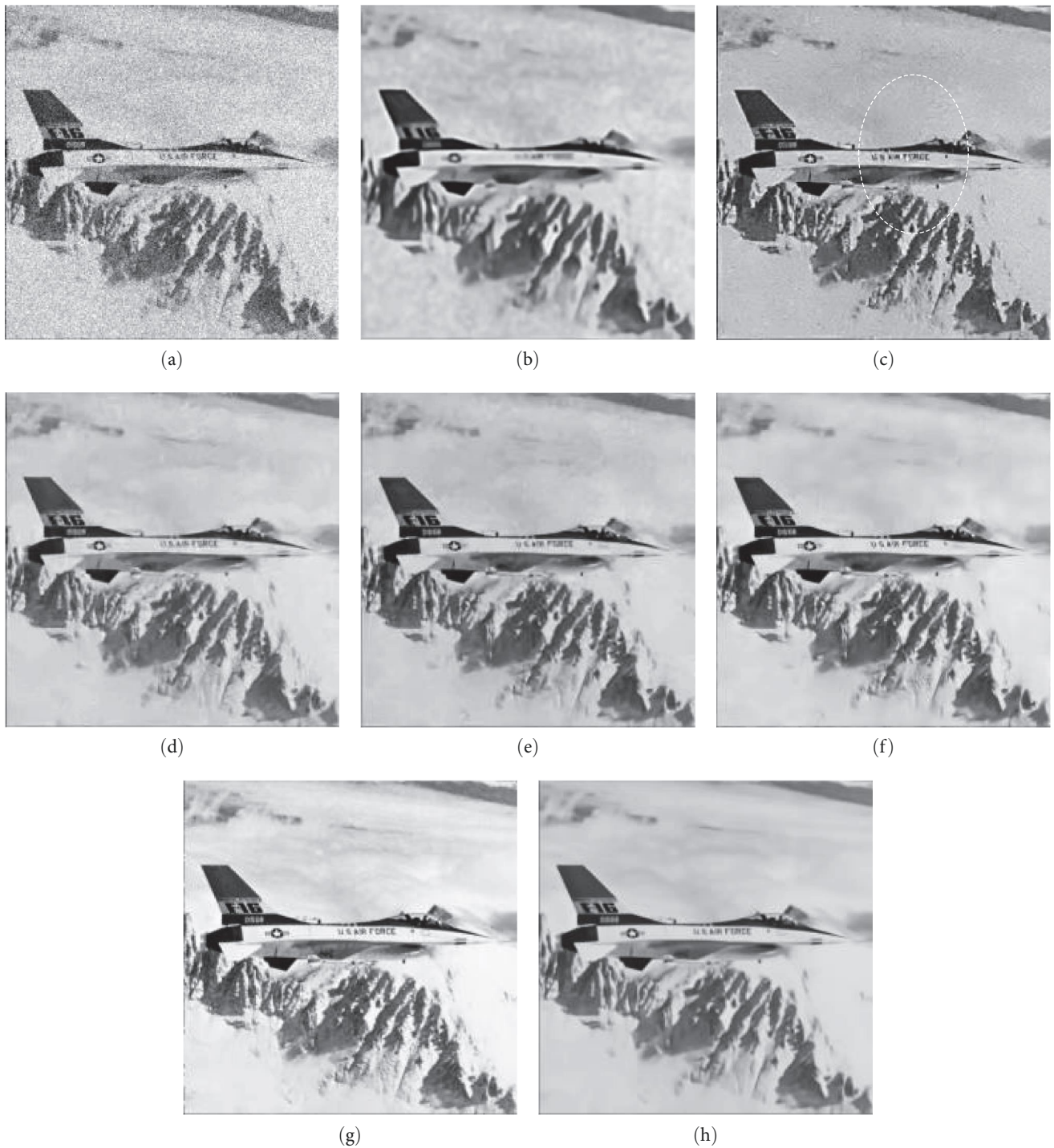
FIGURE 8: Noisy images and denoising results of different algorithms (jetplane): (a) noise image; (b) traditional NLM denoising results; (c) Gaussian kernel NLM denoising results; (d) literature [12] denoising results; (e) literature [13] denoising results; (f) literature [14] denoising results; (g) literature [15] denoising results; (h) denoising results of this paper's method.
