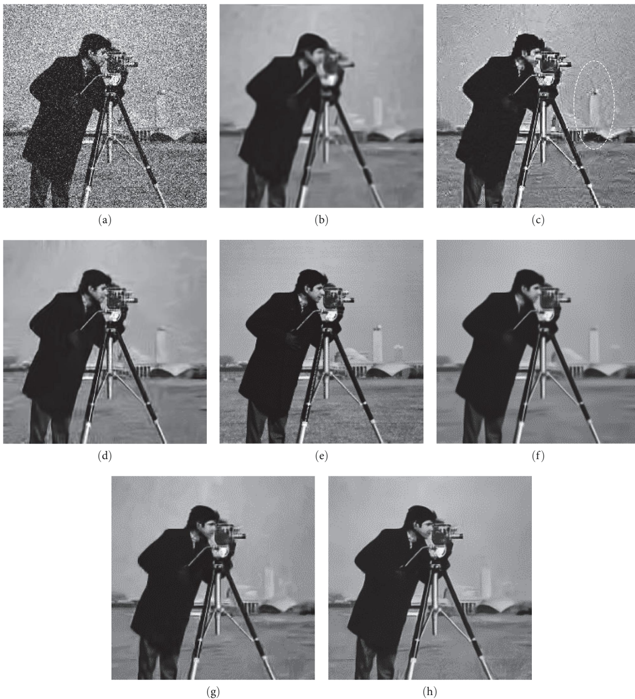
FIGURE 9: Noisy images and denoising results of different algorithms (C.man): (a) noise image; (b) traditional NLM denoising results; (c) Gaussian kernel NLM denoising results; (d) literature [12] denoising results; (e) literature [13] denoising results; (f) literature [14] denoising results; (g) literature [15] denoising results; (h) denoising results of this paper's method.
