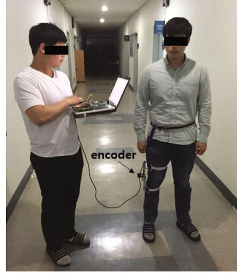
FIGURE 9: Measuring system of the knee motion.
