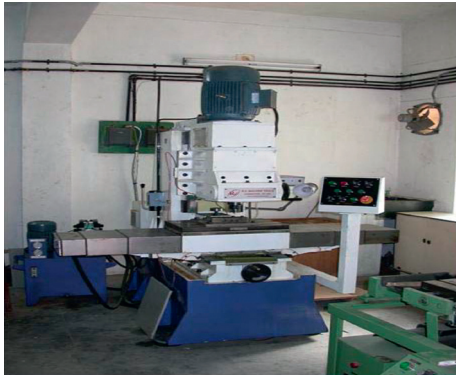
FIGURE 4: Friction stir welding.
