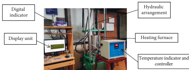
FIGURE 8: Time-dependent creep experimental test equipment.
