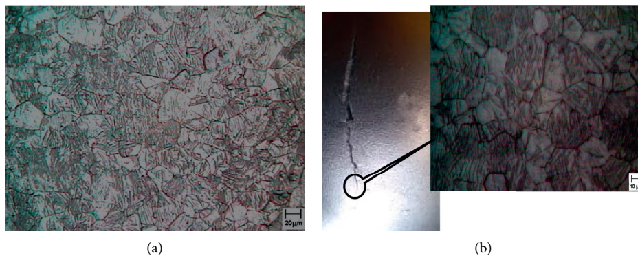
FIGURE 6: Microstructural changes in CP-Ti sample before and after deformation. (a) Original microstructure. (b) Deformed microstructure.
