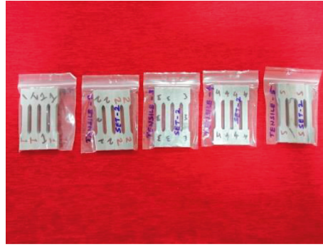
FIGURE 7: Creep test samples as per ASTM standard.
