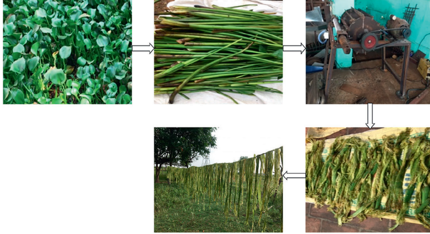
FIGURE 1: Extraction process of water hyacinth plant fibres.
