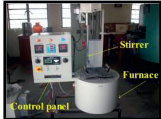
FIGURE 2: Bottom pouring stir casting.
