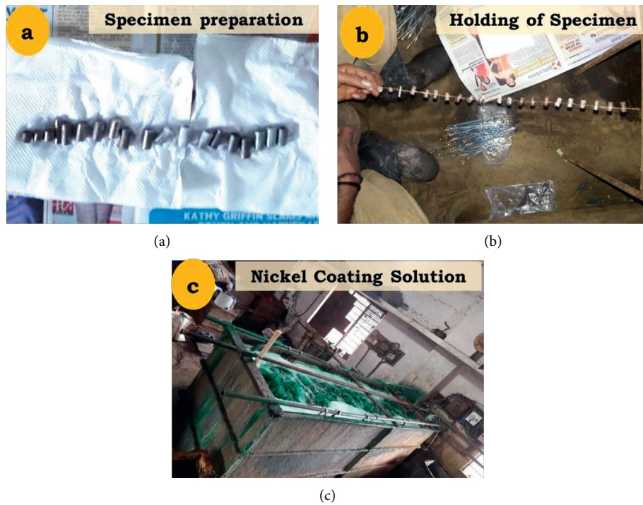
FIGURE 2: Nickel coating of EN8 pin. (a) Specimen preparation, (b) holding of specimens, and (c) nickel sulfate solution.
