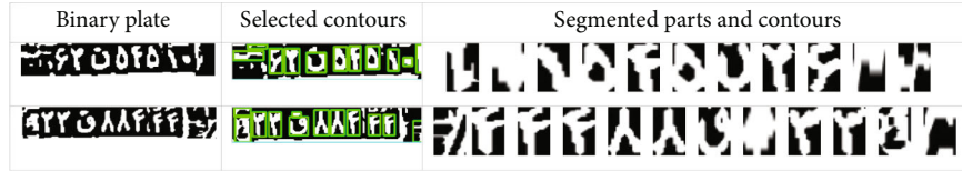
FIGURE 2: General steps of the vehicle plate recognition and detection system.
