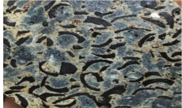
FIGURE 6: Internal structure of nanocoated OPS concrete.
