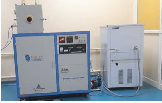
FIGURE 1: Sputtering machine.
