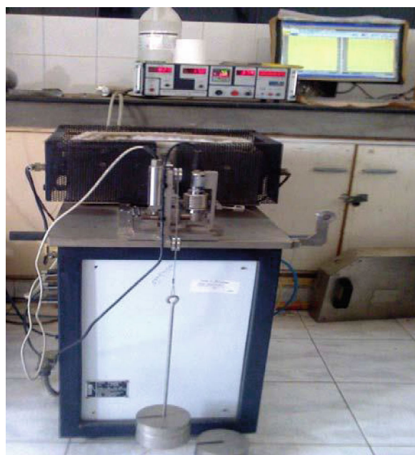
FIGURE 2: Pin on Disc wear testing machine.
