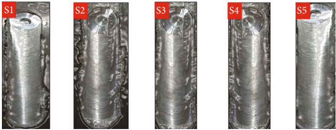
FIGURE 3: FSW interlock weldments joined at varying wt% of nano-SiC.
