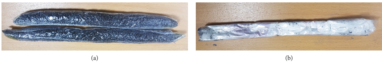
FIGURE 5: Additives to the PV panel between its backside and the installed fins: (a) HDPE grain wraps and (b) folded plastic bags.
