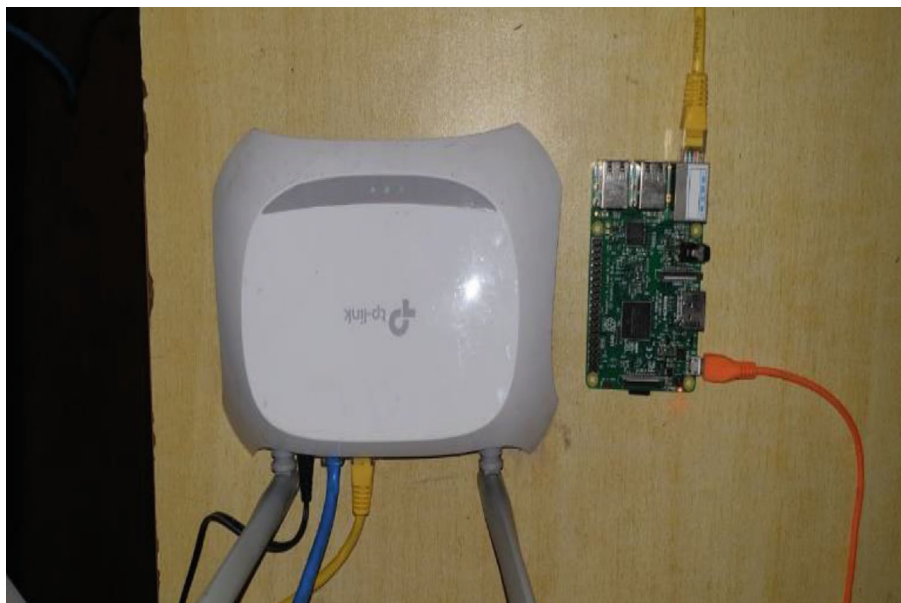
FIGURE 9: Raspberry Pi server and router setup.
