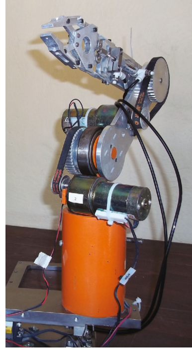
FIGURE 5: Actual 3-DoF anthropomorphic robot arm parameter model.
