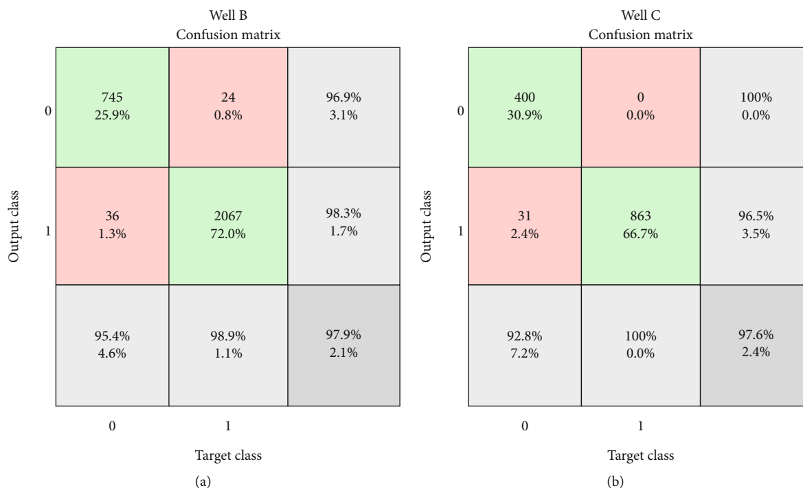
FIGURE 21: Confusion matrix for the prediction of lost circulation zones in Well B (a) and Well C (b) using the ANN technique.
