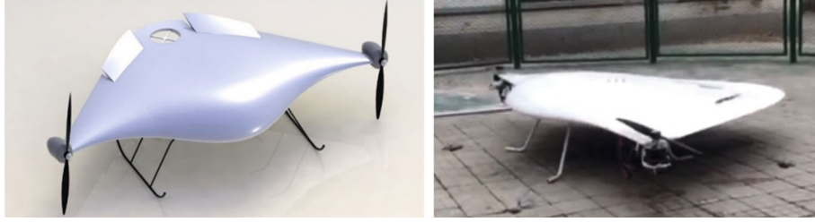
FIGURE 1: The tiltrotor aircraft studied in this paper.
