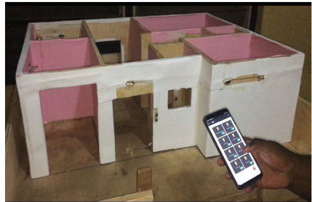
FIGURE 21: Demo house with all LEDs, motors, and sensors integrated.
