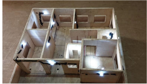
FIGURE 19: Constructed demo house with LEDs integrated.
