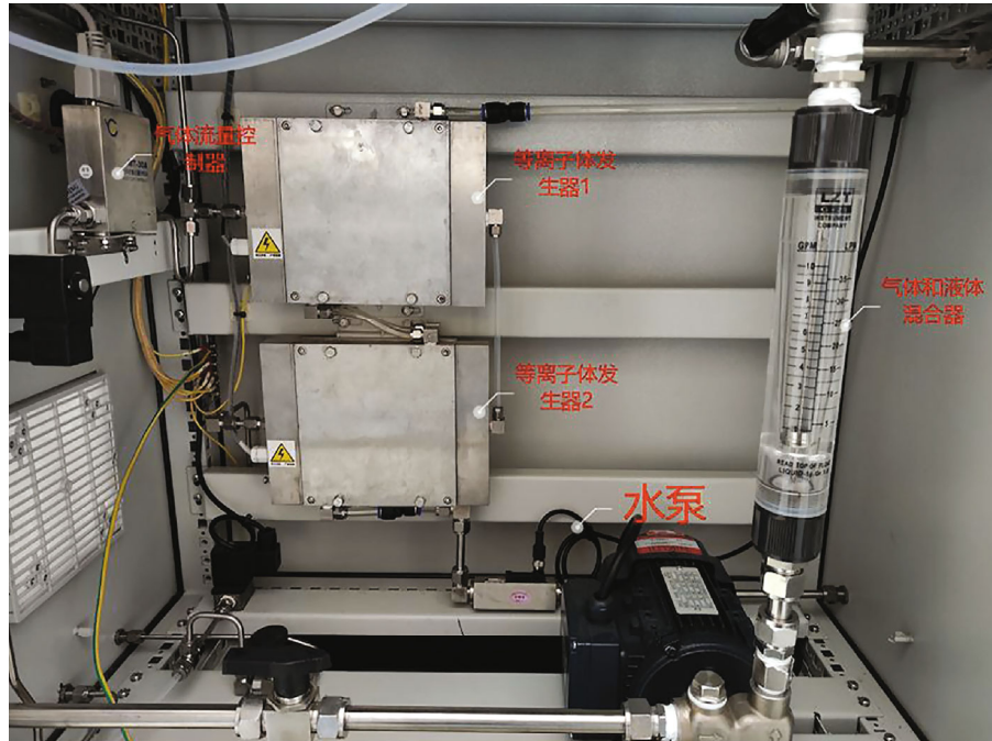
FIGURE 7: Plasma reactor.
