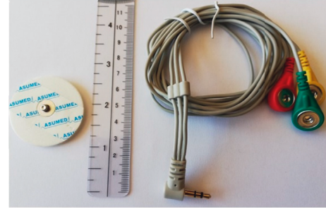
FIGURE 2: Example view of electrodes and shielded cables.
