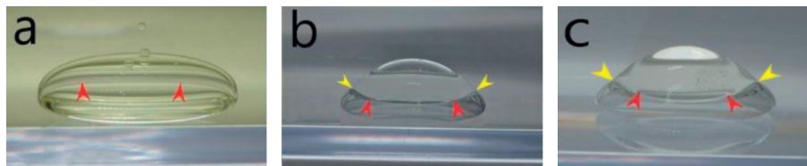
FIGURE 3: Shape of each immiscible droplet exhibiting a smooth surface. The shape of each immiscible droplet exhibiting a smooth surface is shown (the red arrowheads indicate the border between two materials). Silicone oil-perfluorooctane immiscible droplet in canola oil (upper: silicone oil, lower: perfluorooctane) (a), silicone oil-perfluorooctane immiscible droplet in aqua (upper: silicone oil, lower: perfluorooctane) (the yellow arrowheads indicate the contact point among perfluorooctane, silicone oil, and aqua) (b), and canola oil-perfluorooctane immiscible droplet in aqua (upper: canola oil, lower: perfluorooctane) (the yellow arrowheads indicate the contact point among perfluorooctane, canola oil and aqua) (c).
