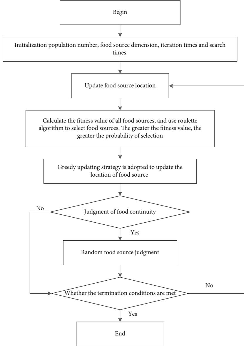
FIGURE 2: Flow chart of artificial bee colony algorithm.
