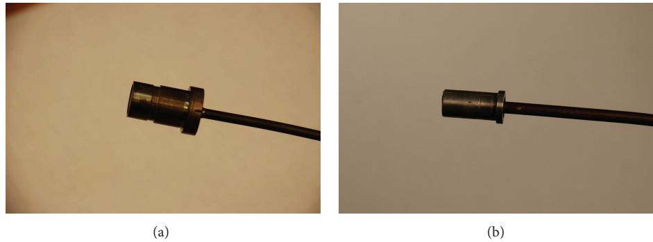
FIGURE 1: Microwave blade tip clearance probe (Meggit). (a) 5.8 GHz probe. (b) 24 GHz probe.
