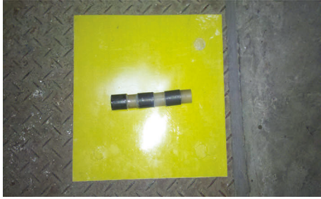
FIGURE 6: Phononic crystal is composed of steel and silicone rubber.
