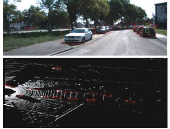
FIGURE 1: Detection results for Pointpillar.
