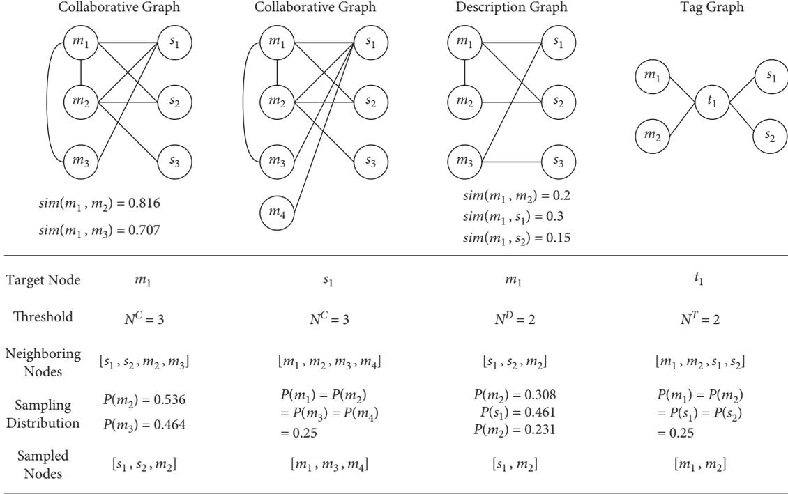
FIGURE 3: An illustration of the node sampling process.
