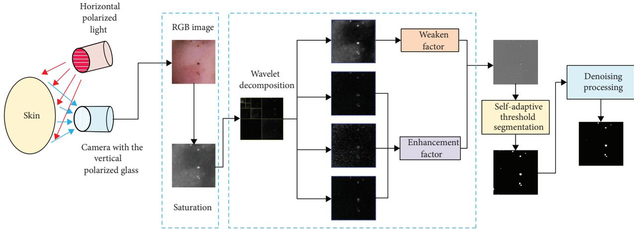
FIGURE 1: The schematic diagram of the proposed method.
