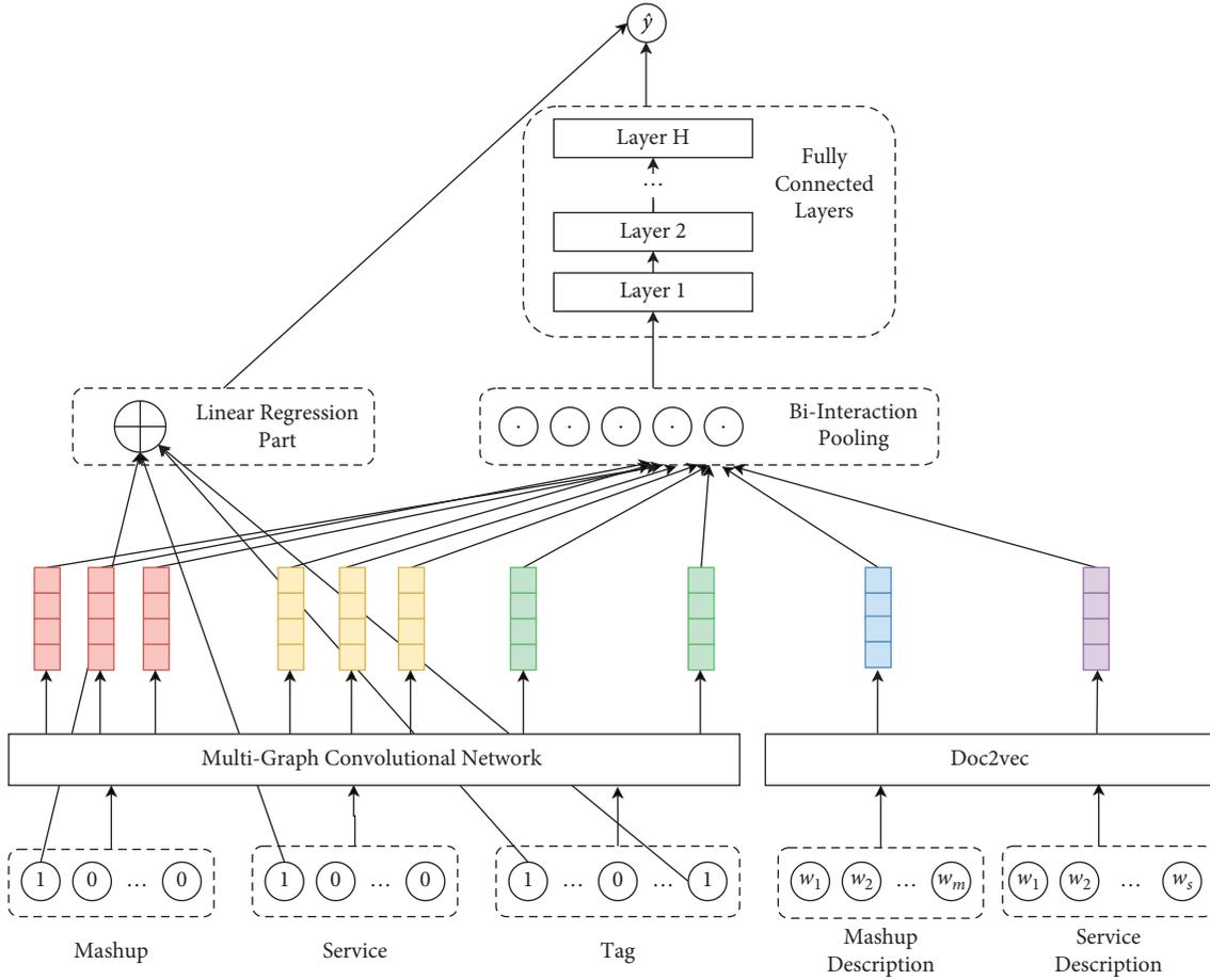
FIGURE 4: A framework of the neural factorization machine model.
