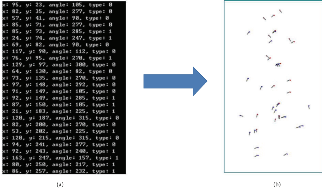
FIGURE 11: Restored minutiae points and their graphical representation using x , y , and \theta (reproduction of Figure 2 in [19]).
