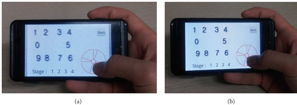
FIGURE 4: Implementation of 3DPIN (reproduction of Figure 2 in [8]). (a) Case wherein the camera sees blurred digits. (b) Case wherein the camera sees only one image.
