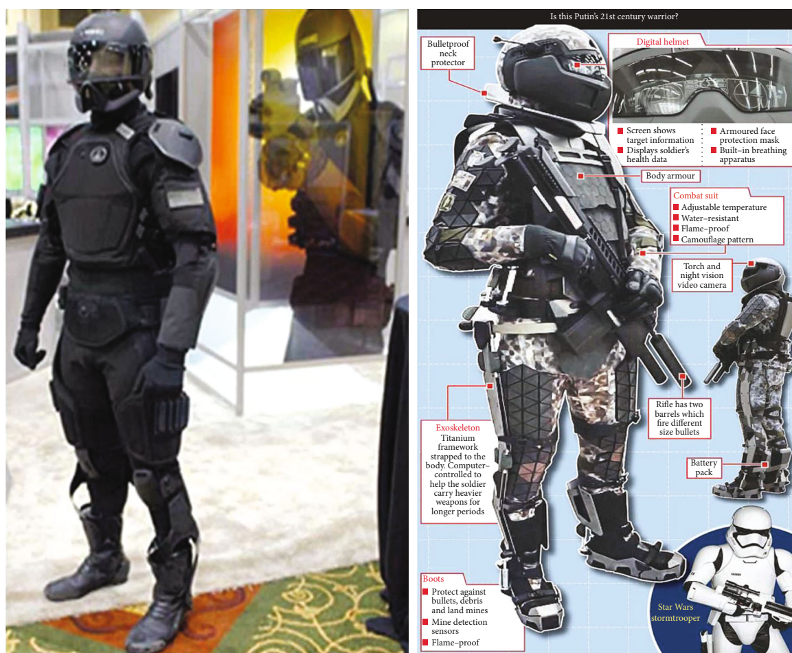
FIGURE 5: Russian advanced high-tech amour item that includes an exoskeleton or the outer layer, designed to boost strength and stamina [67].
