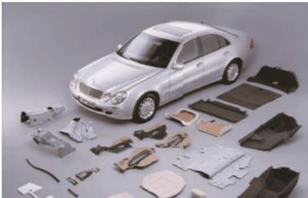
FIGURE 1: A vehicle showing numerous parts produced from PMCs [36].
