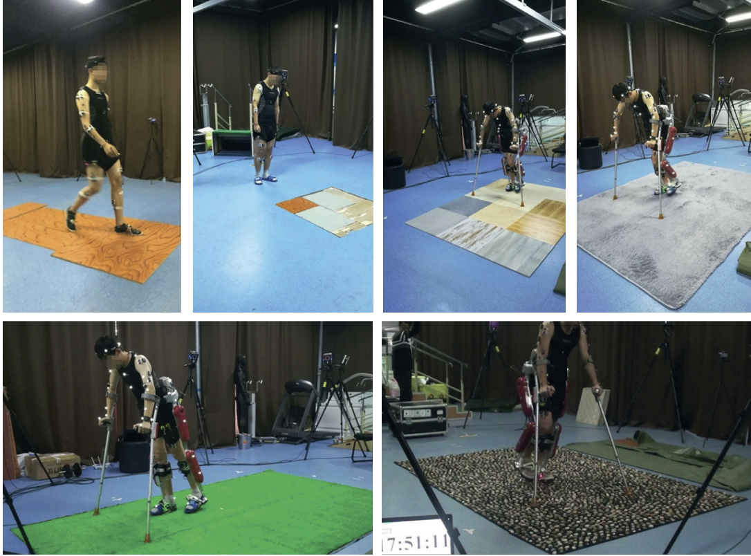
FIGURE 1: Experimental setup and walk test. The subjects walk on flat floors with 6 different friction situations with and without exoskeletons. Their gait information is acquired by motion capture devices and sensors.
