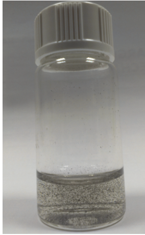
FIGURE 2: Appearance of the dispersion composed of carbon nanotubes (CNTs) mixed with saline solution in which concentration is 1 mg/mL.
