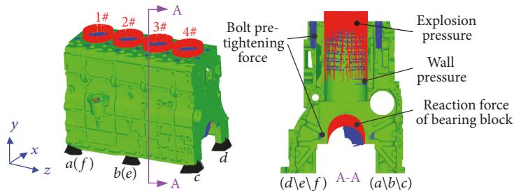
FIGURE 3: The loads and boundary conditions of cylinder block.
