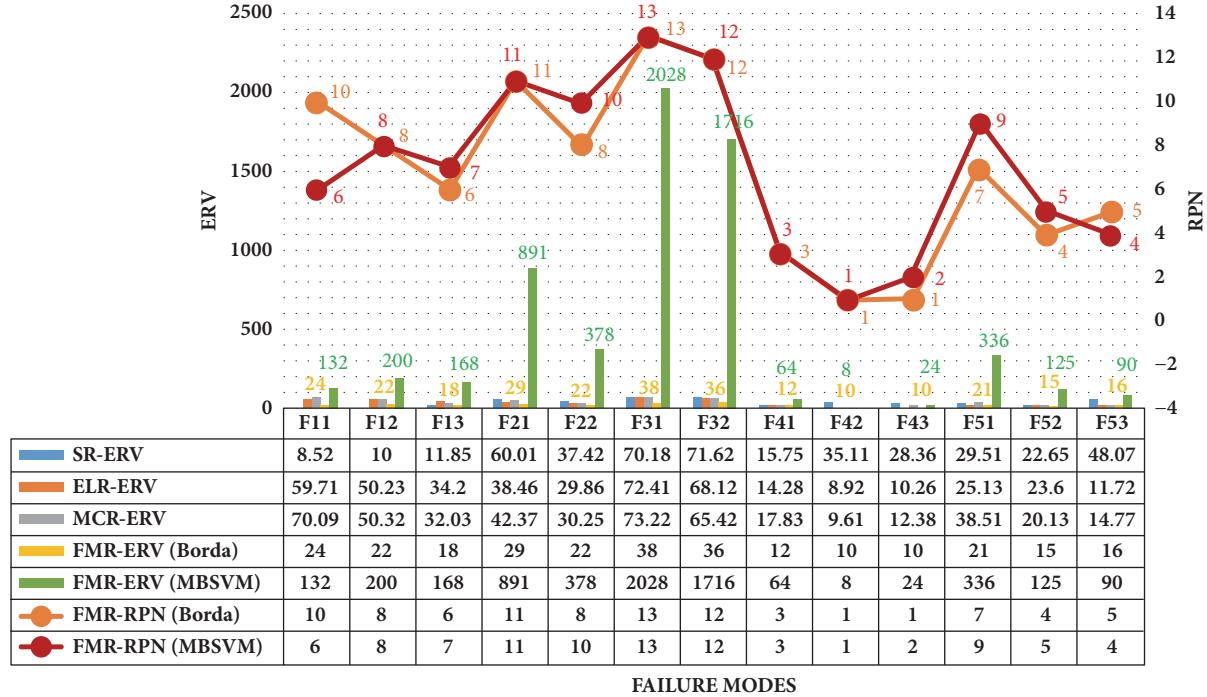
FIGURE 6: ERV and RPN of integrated risk of each failure mode with traditional Borda and the MLBM.
