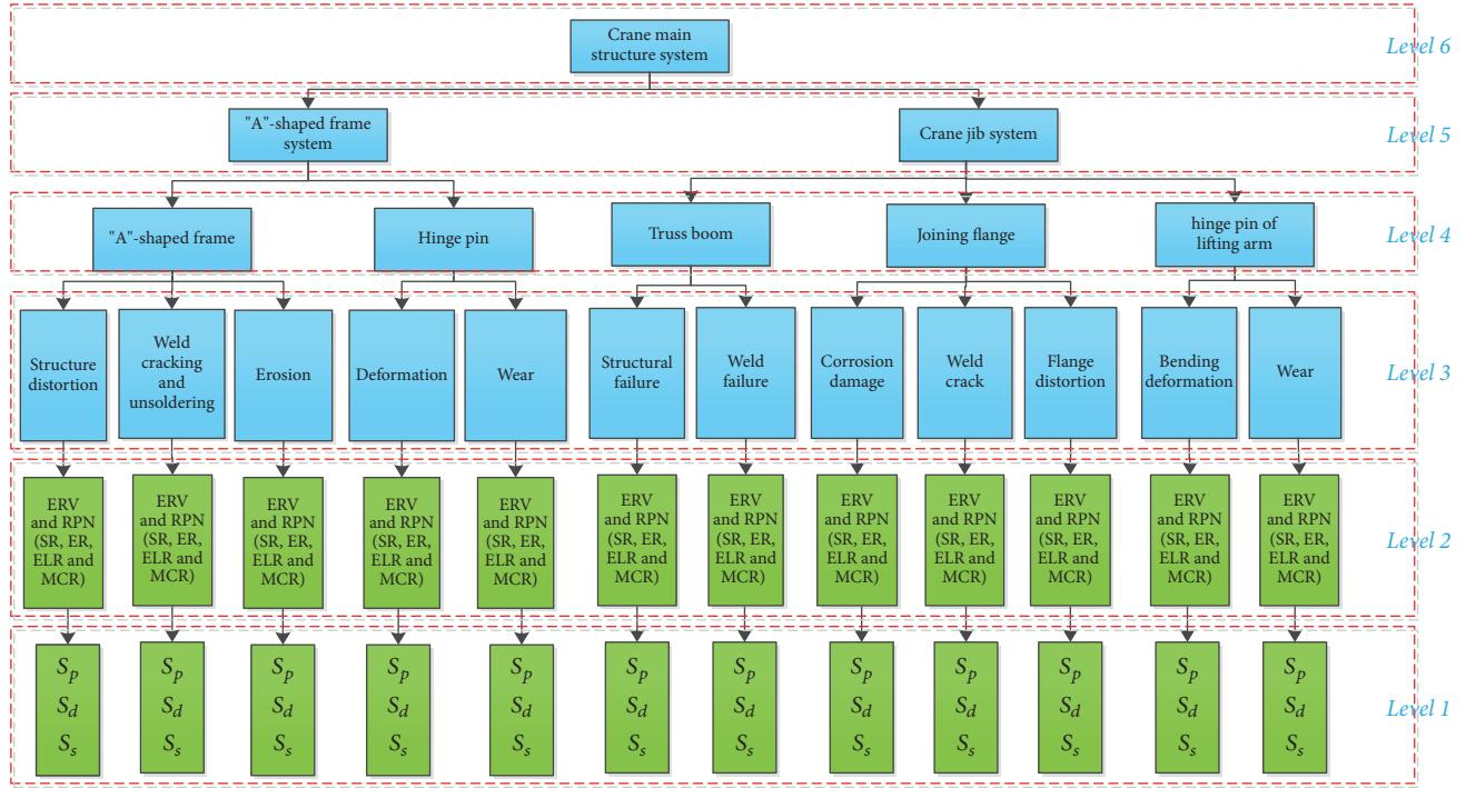
FIGURE 4: The RHT of the main structure system of the truss type crane.
