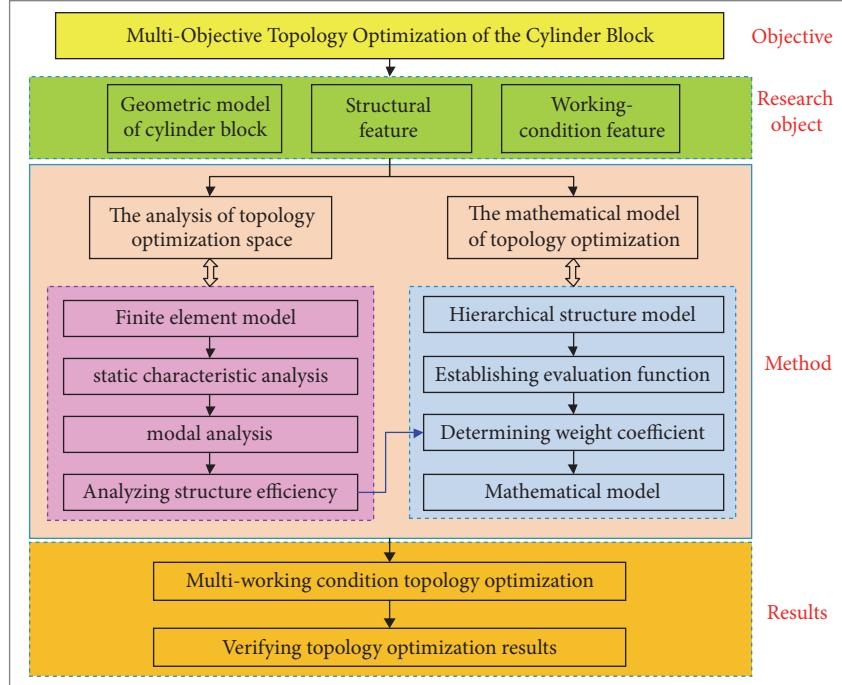
FIGURE 1: The block diagram of multiobjective topology optimization.
