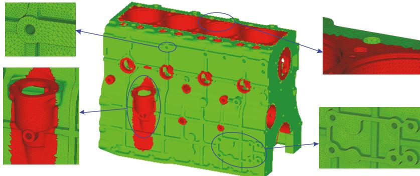
FIGURE 4: The finite element model.
