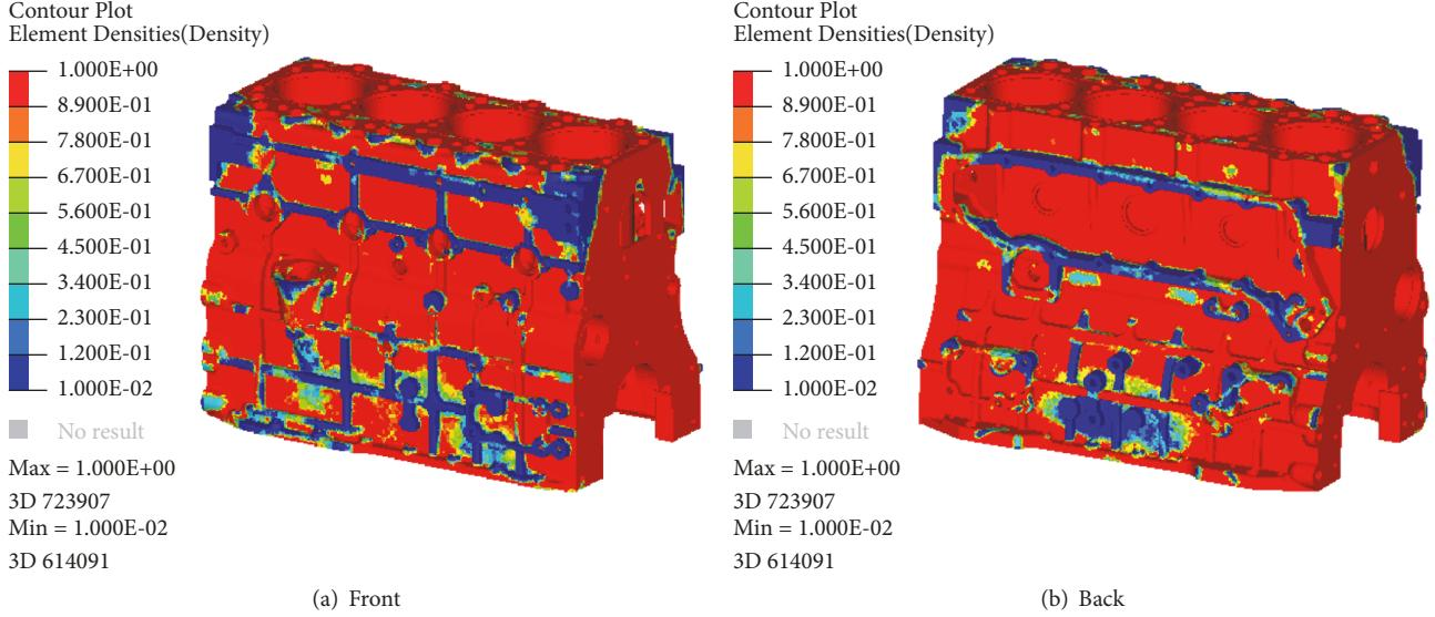
FIGURE 12: Result of the multiobjective topology optimization.
