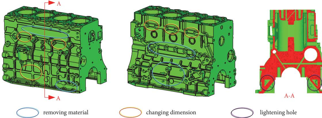
FIGURE 13: New model of the cylinder block.
