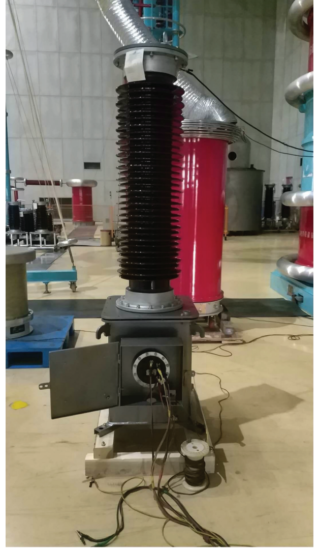
FIGURE 4: Test platform of the CVT.
