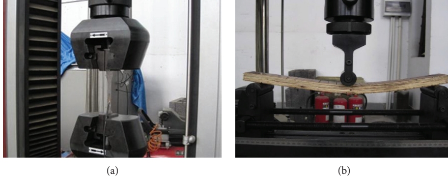
FIGURE 1: Test of material properties. (a) Test for steel sheet. (b) Test for bamboo plywood.
