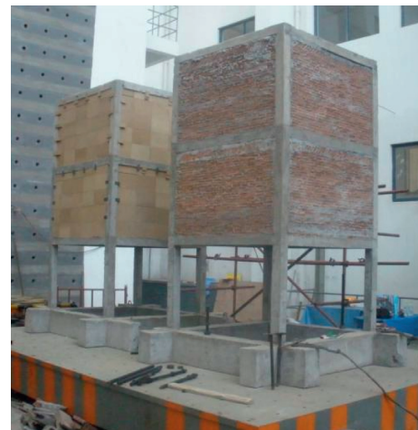
FIGURE 8: Test structures on shaking table.
