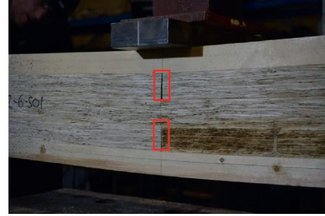
FIGURE 1: Butt joints in the 2 nd and 4 th layer of a 5-layer A1a specimen.
