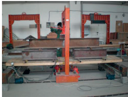
FIGURE 7: Eight points bending test. (a) Diagrammatic view. (b) Photograph.
