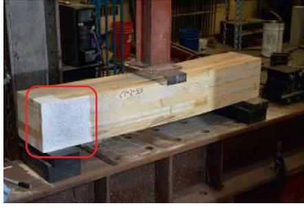
FIGURE 2: DIC area in shear test and related shear diagram.
