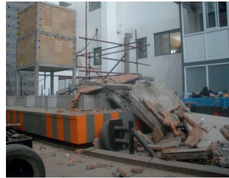
FIGURE 13: Crumble of the brick frame.
