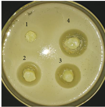
FIGURE 8: The cellulose/ \beta -CD hydrogel with different concentrations of \text{TiO}_2 .
