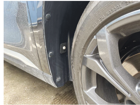
FIGURE 2: The humidity sensor behind a car tire.
