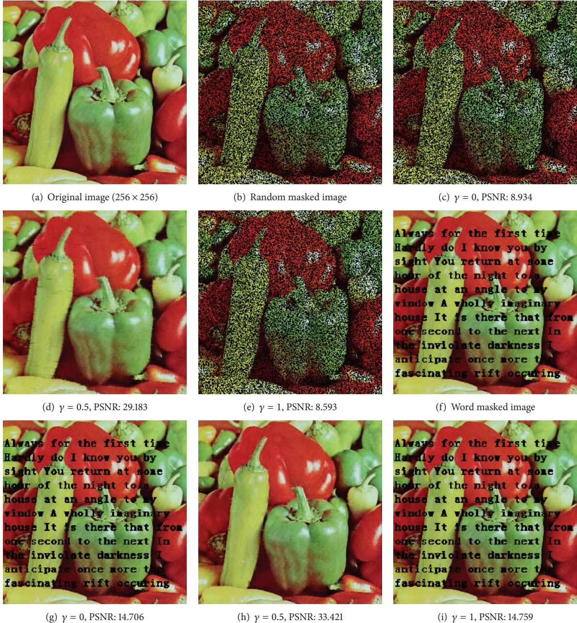
FIGURE 1: The recovered results with 60% random mask and word mask for \gamma = 0, 0.5 and 1 by LTVNN.
