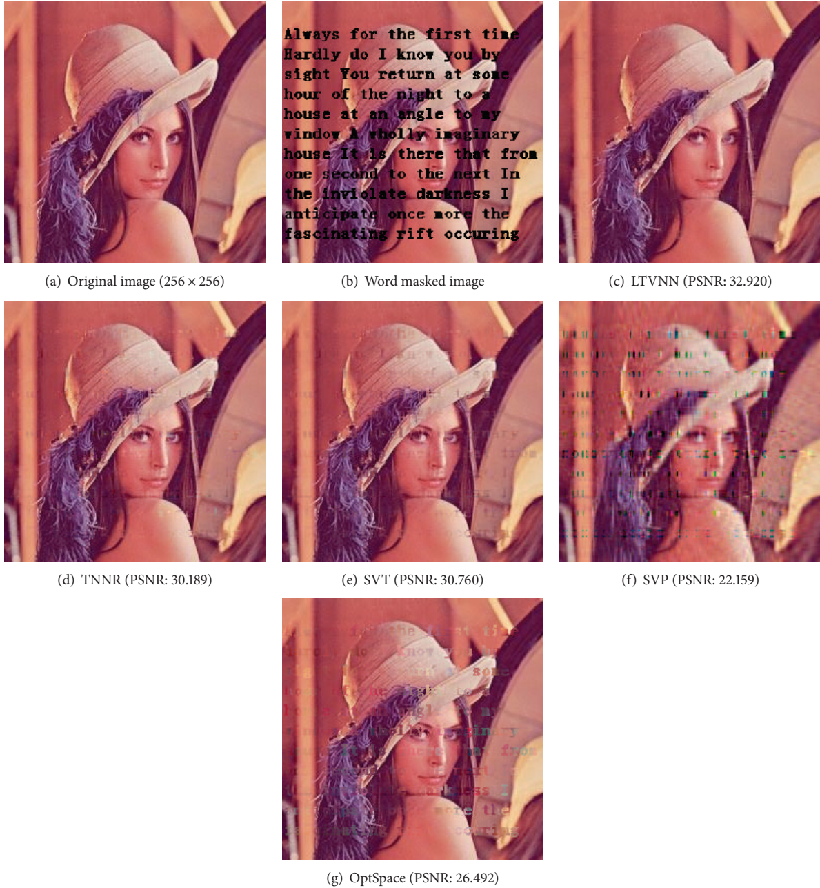
FIGURE 4: Comparison of PSNR of recovered methods for Lena under word mask with \gamma = 0.5 by LTVNN, TNNR, SVT, SVP, and OptSpace.
