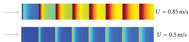
FIGURE 2: Axial variation in local interphase mass transfer coefficient.
