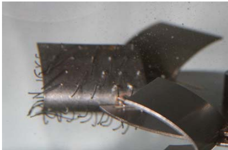
FIGURE 9: Telltales on BT-6 impeller blade.
