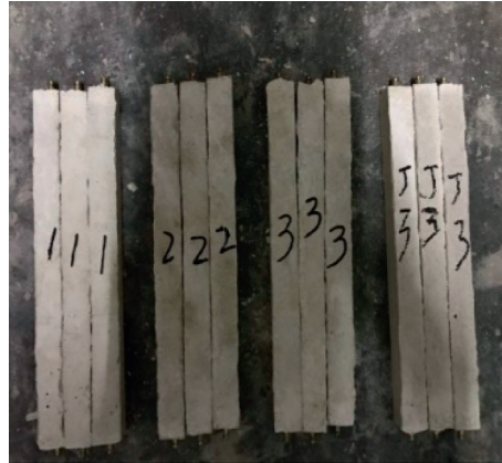
FIGURE 3: Preparation of drying shrinkage test specimen.
