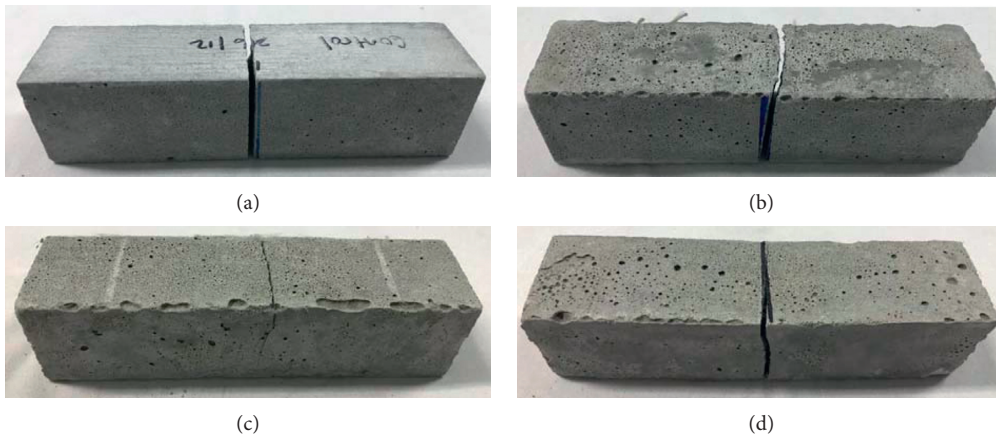
FIGURE 7: Fractured LCC after 3-point bending test: (a) control mix; (b) LCC-basalt; (c) LCC-PVA; (d) LCC-PP.
