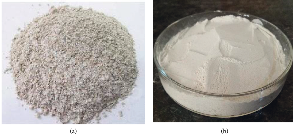
FIGURE 3: Identified industrial waste GBFS before and after milling: (a) as-received GBFS and (b) milled GBFS.
