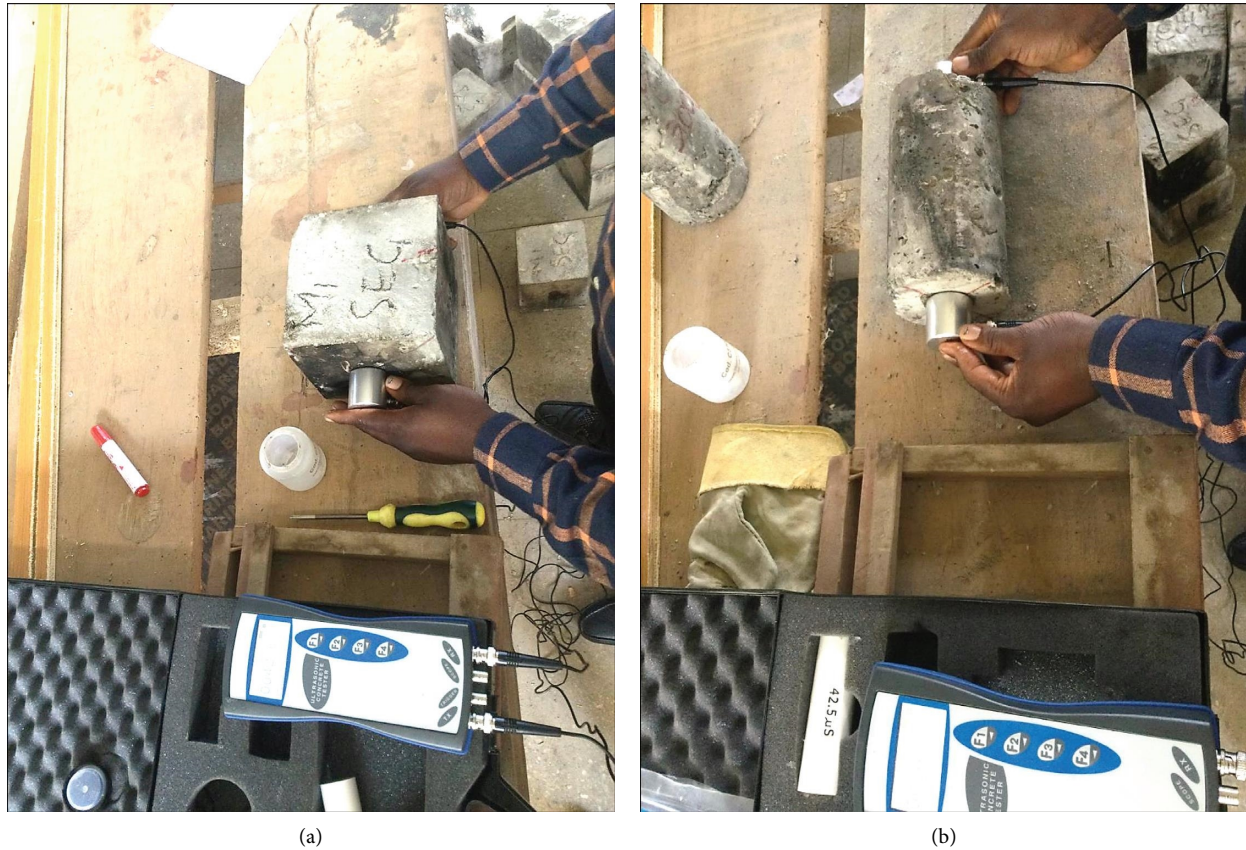
FIGURE 7: Ultrasonic pulse velocity test on hardened concrete cube and cylinder.
