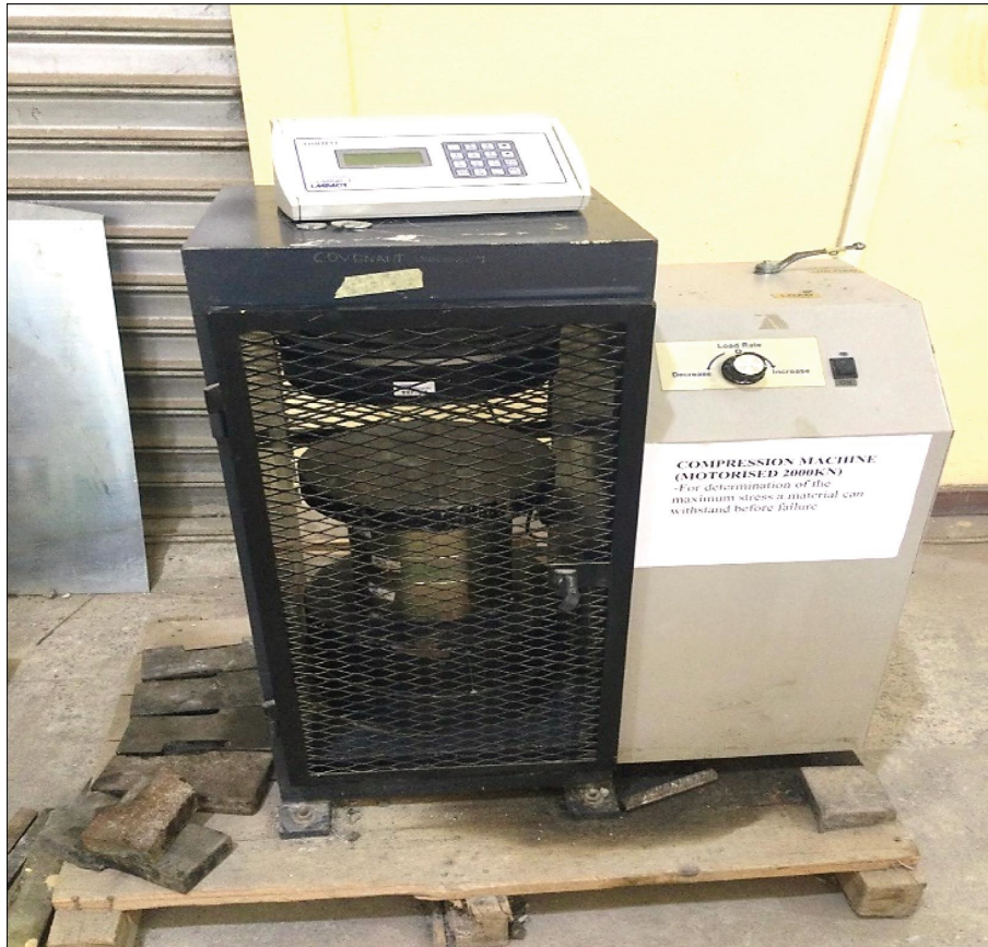
FIGURE 3: Compressive strength machine.
