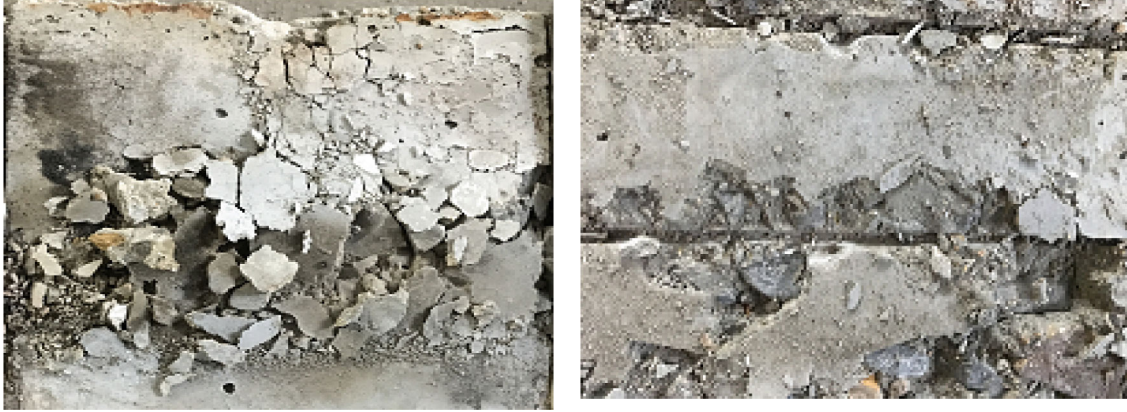
(a) Damage of concrete in B0
