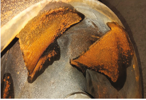
FIGURE 1: Cavitation erosion in the centrifugal pump.
