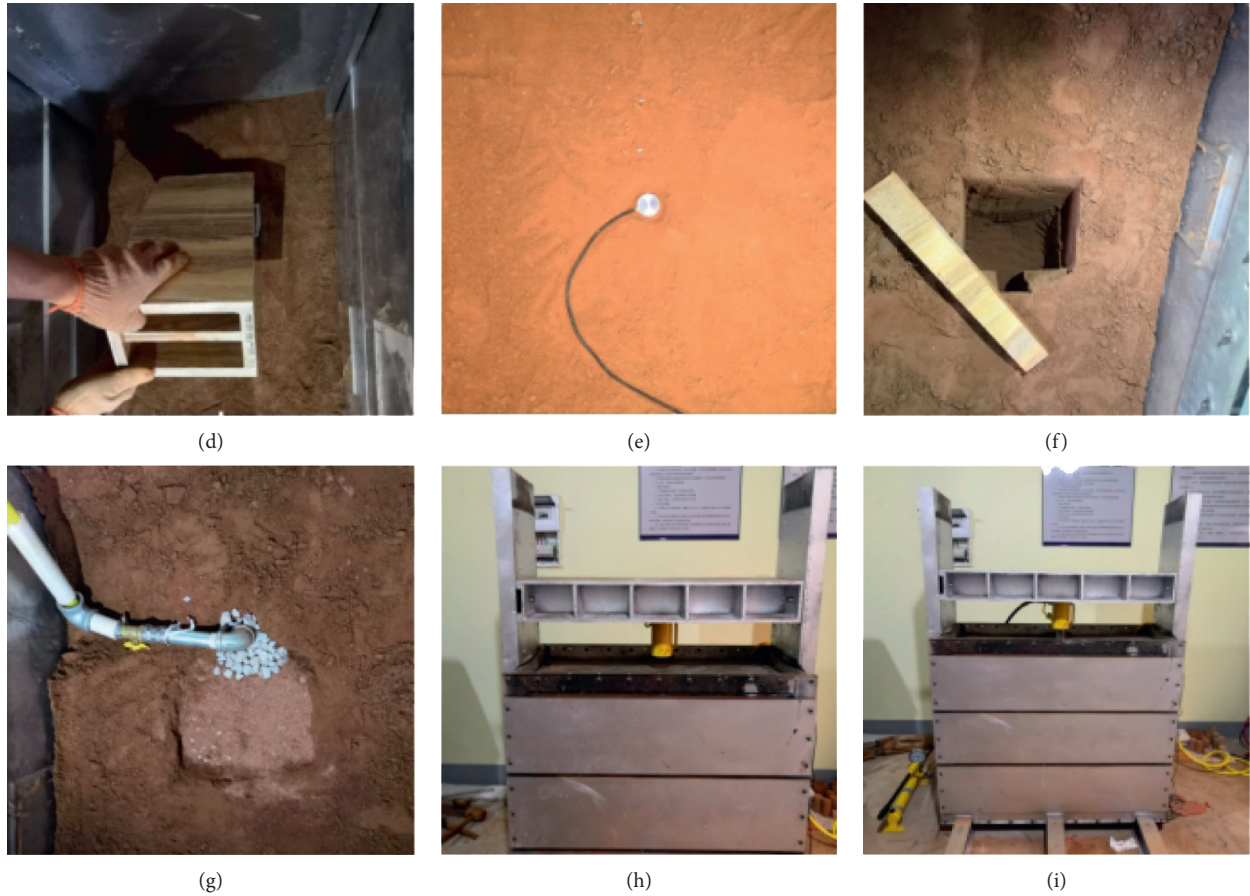
FIGURE 8: Model body production process. (a) Embedded glass panel. (b) Filling materials. (c) Layer compaction. (d) Mold positioning. (e) Embedded monitoring elements. (f) Molding. (g) Filling fault buried water pipe. (h) Install reaction frame and jack. (i) Hydraulic loading.
