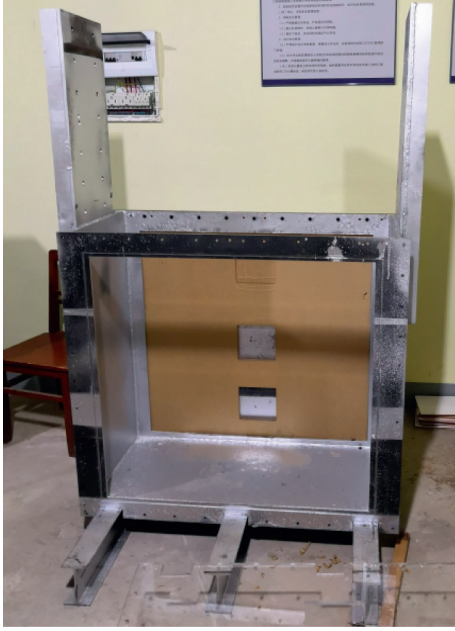
FIGURE 1: Main structure of the test frame.
