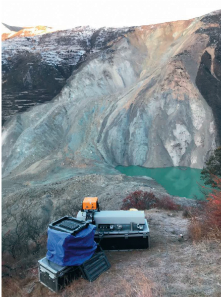
FIGURE 4: Field monitoring photos of the slope radar.
