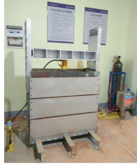
FIGURE 5: Tunnel water and mud inrush fluid-solid coupling 3D visualization physical model test system.
