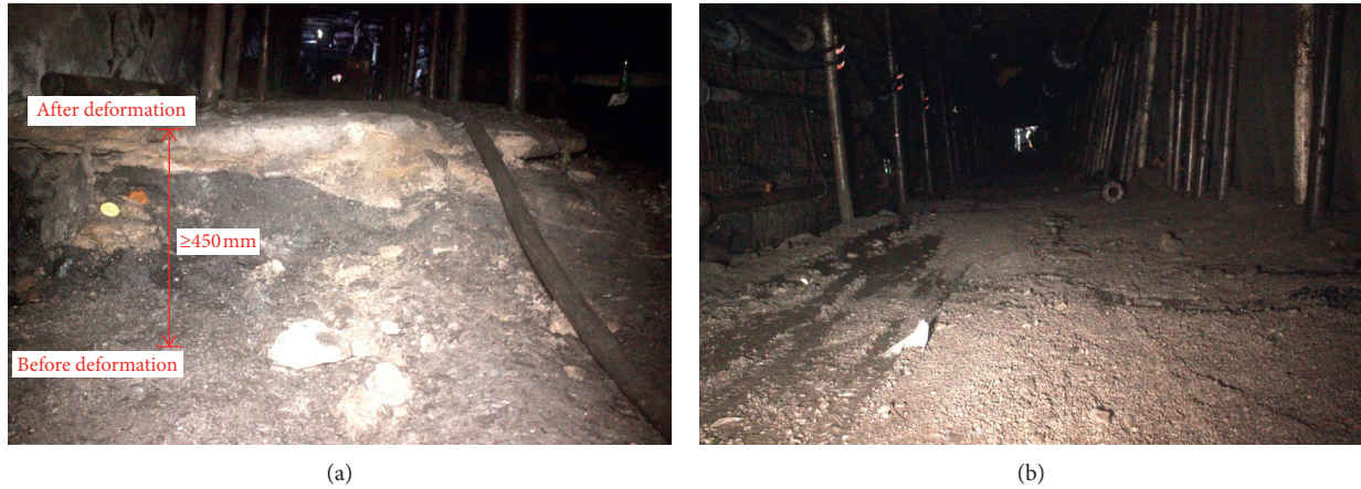
FIGURE 20: The control effect on floor heave. (a) Before control. (b) After control.
