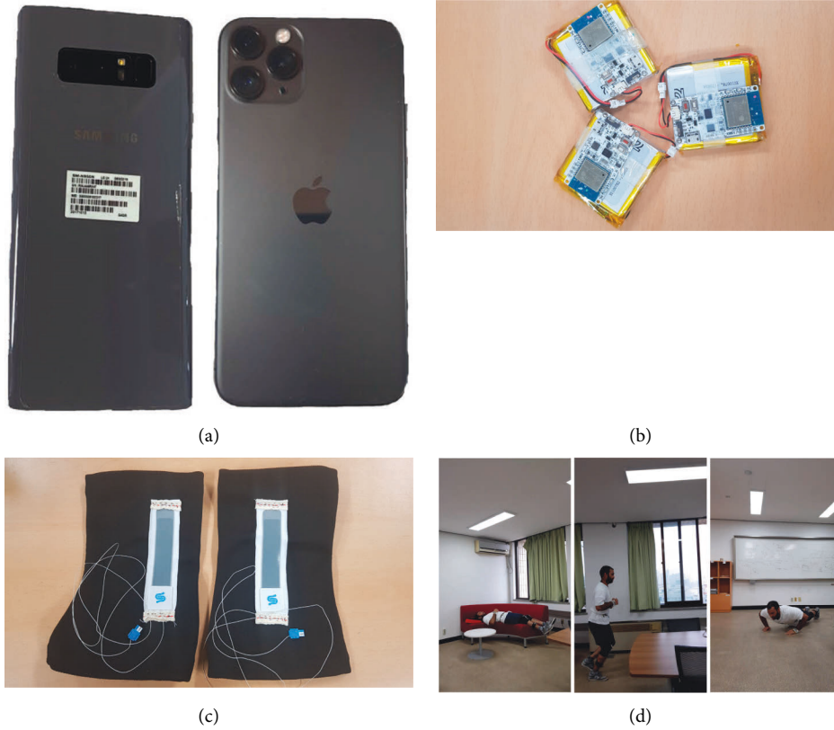
FIGURE 6: Experiment setup. (a) Smartphones. (b) IMU sensor. (c) Stretch sensor. (d) Experiment area.
