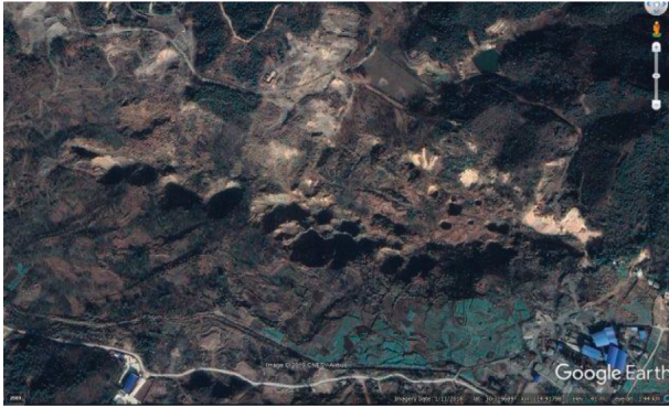
FIGURE 2: Subsidence features at China's Chengchao iron ore mine. Image courtesy of Google Earth, taken in 2018.
