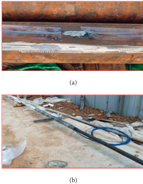
FIGURE 7: Steel pipe pile and anchor sensor installation. (a) Installation of FBG strain sensor. (b) Installation of FBG axial force sensor.
