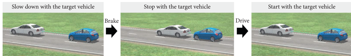
FIGURE 11: The vehicle autonomous stop-and-go task in CARSIM.
