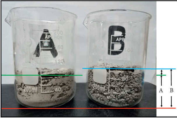
FIGURE 1: Volumetric testing of coarse-grained and fine-grained mixtures.
