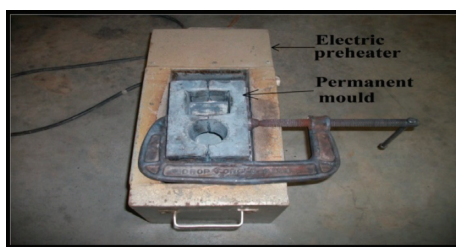
FIGURE 2: Preheater of the permanent mould.
