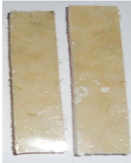
FIGURE 10: Specimen for impact test.
