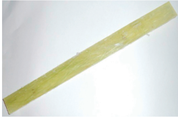
FIGURE 9: Specimen for flexural test.
