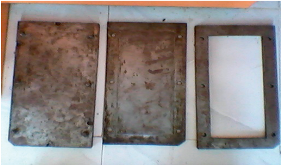
FIGURE 7: Steel die mold.
