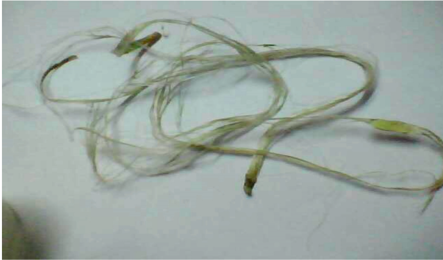
FIGURE 3: Extracted mudar fiber.
