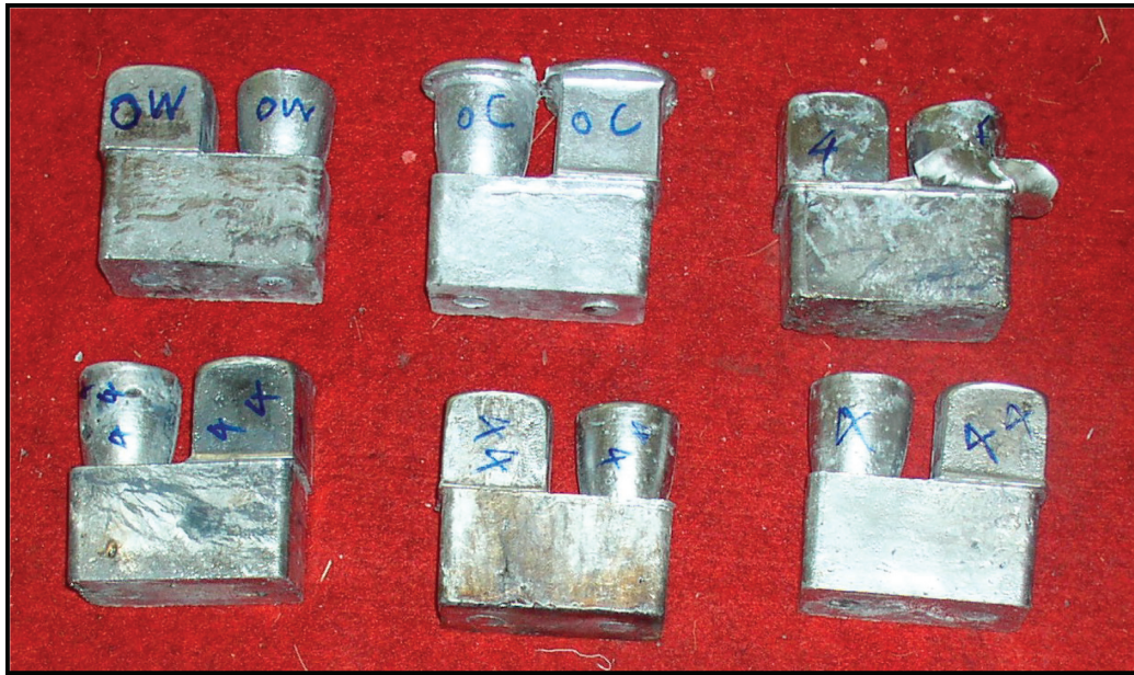
FIGURE 3: Fabricated AA6061/Si 3 N 4 composite castings.
