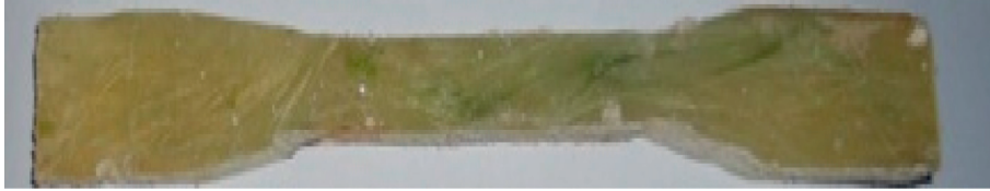
FIGURE 8: Specimen for tensile test.
