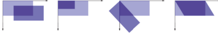
FIGURE 2: Four basic transformation types: translation, scale, rotation, and skew.
