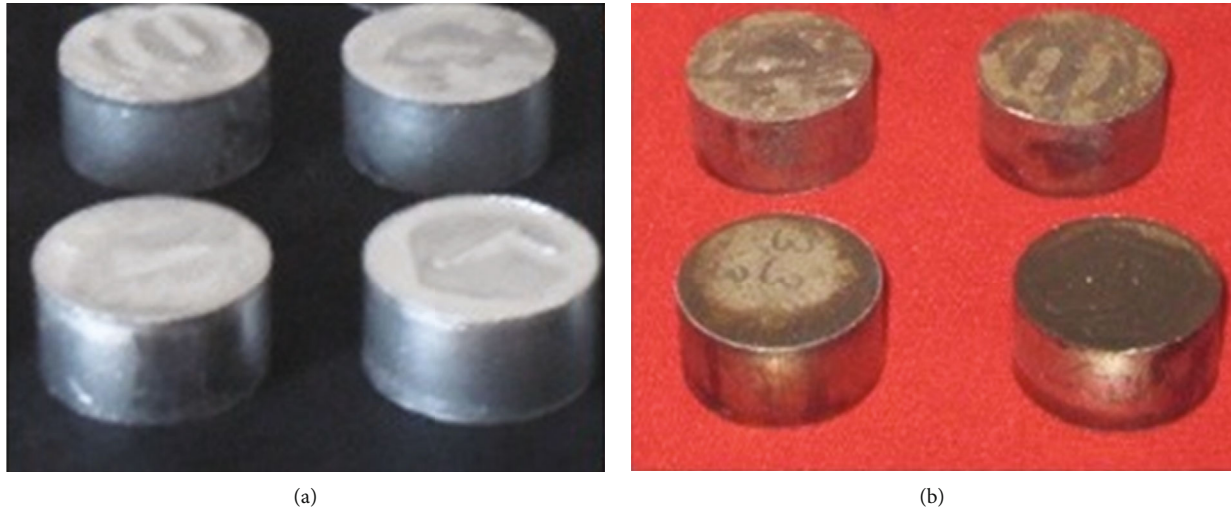
FIGURE 3: Compacted billets (a) before sintering and (b) after sintering.
